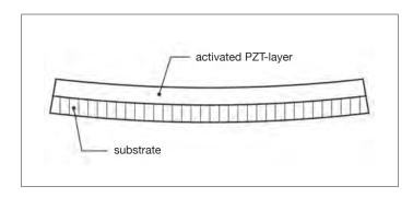
Fig. 18 c: Bending structure by gluing a PZT-layer onto a thin substrate.
