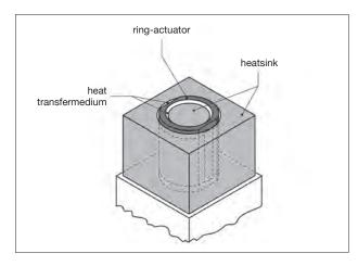
Fig. 13: Scheme of highly efficient ring-actuator cooling by inner and outer heat-sinking
