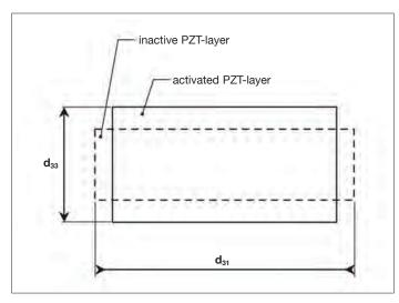
Fig. 18 a: Action of a free PZT-layer
