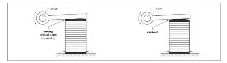
Fig.17 c: Incorrect/correct coupling of a rotating mechanism
