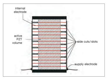
Fig. 9: Isi-based stack with stress relaxation side slots
