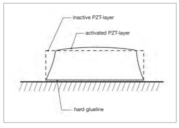
Fig. 18 b: Hindered expansion of a PZT-layer by clamping by a hard glue line together with a rigid substrate
