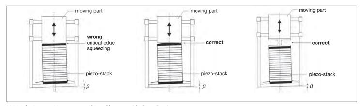
Fig. 17 b: Incorrect/correct coupling of linear guided mechanics
