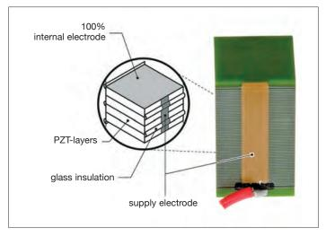
Fig. 2: Schematic of the osi-technique using fused-on glass fibers to terminate internal electrodes on stack's surface
