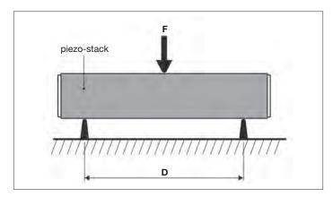
Fig. 4: Schematic of a bending experiment
