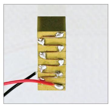
Fig. 8: Chip-based piezo-stack
