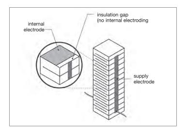
It is easily seen, that the PZT-ceramic of the stack is only partially active and a steep transition from active to inactive PZT-ceramic is created: A pronounced mechanical tensile stress at the active/inactive boundary region occurs, when the PZT-stack is activated and expanding (Fig. 7). internal
