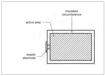
Fig. 11: "Buried electrode" scheme
