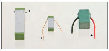
Fig. 20: Actuator's poling
