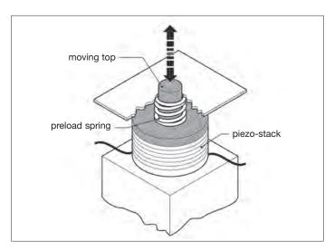
Fig. 15:Schematic of a preload spring mechanism
