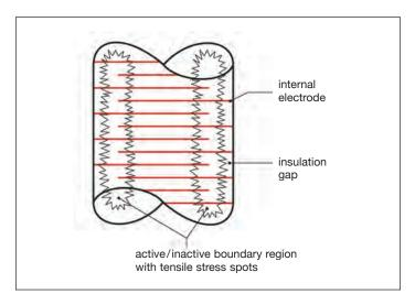
Fig.7: Mechanical stress generation inside a isi-piezostack at the active/inactive boundary
