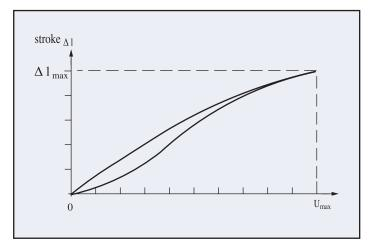
Fig 27a: Voltage/stroke relation
