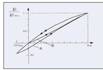
Fig. 9: Normalized stroke/voltage diagram of standard high voltage stacks PSt 500 and PSt 1000 A. For bipolar operation in the range  $(-)0.2 U_{max}$  thru  $(+)U_{max}$ B. For unipolar operation in the range 0 V thru  $(+)U_{max}$
