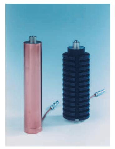
Fig. 20: Different configurations for the heat management of actuators using the "ThermoStable" technique. Left side: actuator with copper casing for heat sinking. Right side: actuator casing with air cooling fins for forced air cooling.
