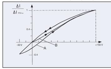
Fig. 8: Normalized stroke/voltage diagram of low voltage stacks (relative stroke 1 for voltage step  $0 \text{ V/U}_{max}$ ) A. For bipolar operation in the range (-)0.2 U<sub>max</sub> thru (+)U<sub>max</sub> B. For unipolar operation in the range 0 V thru (+)U<sub>max</sub>
