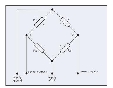
*Fig. 17: Schematic of a Wheatstone bridge configuration of strain gauges for position detection*
