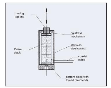
Fig. 3: Schematic of an actuator with prestress
