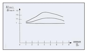
*Fig.14: Strain enhancement upon prestress for different PZT materials.*
