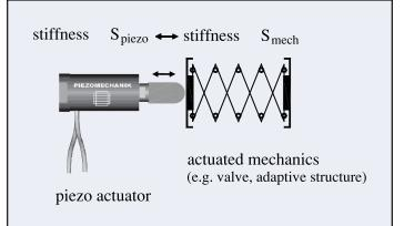
Fig. 4: Schematic of a piezo actuated system: A piezo actuator interacts with a coupled mechanism, where the piezomechanical performance is defined by the two interacting stiffnesses Spiezo and Smech.
