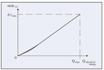
*Fig. 27b: Charge/stroke relation*
