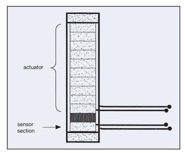
*Fig.*19: *Schematic of an integrated actuator-force sensor configuration*
