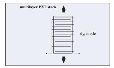
Fig. 1b: Schematic of an axially acting multilayer piezo-stack
