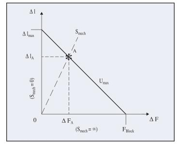
*Fig. 7: Shows a diagram spanned by piezo actuator's max. stroke versus blocking force*
