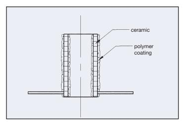
Fig. 2: Schematic of a stacked ring actuator
