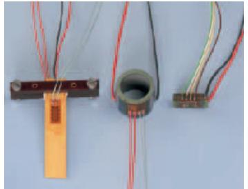
*Fig. 18: Variety of piezoactuating components with surface mounted strain gauges*
