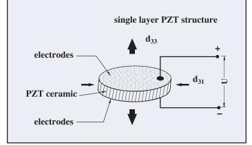
Fig. 1a: Schematic of a piezoelectric single layer element
