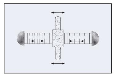
*Fig. 15: Schematic of a bipolar antagonistic actuator system for active resetting.*
