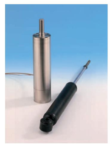
*Fig. 21: Large cross section custom designed actuator for active vibration cancellation, 56 mm diameter for very high loads of 100 kNewtons*
