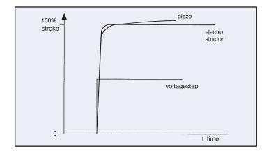
*Fig.12a: Normalized stroke/voltage characteristic for electrostrictive actuators, unipolar operation only.*
