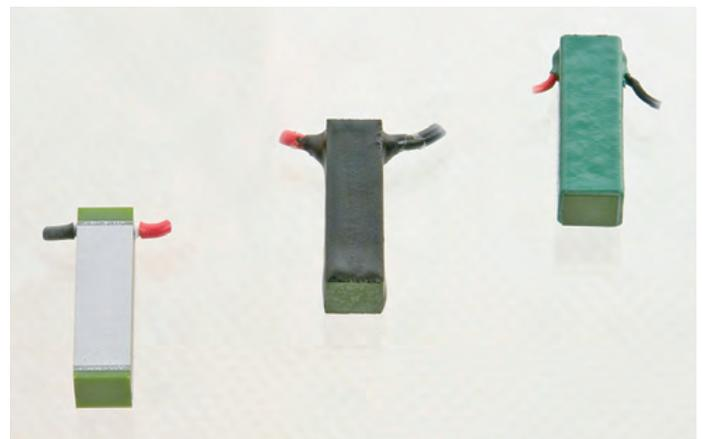
Fig. 3: Different kinds of stack coatings
