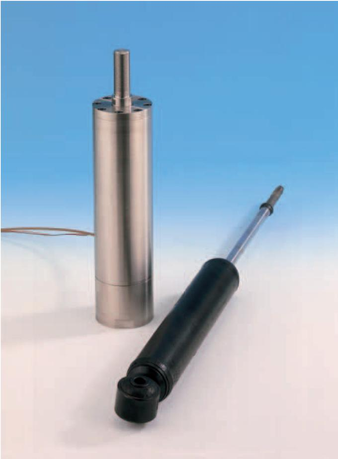
*Fig. 21: Large cross section custom designed actuator for active vibration cancellation, 56 mm diameter for very high loads of 100 kNewtons*
