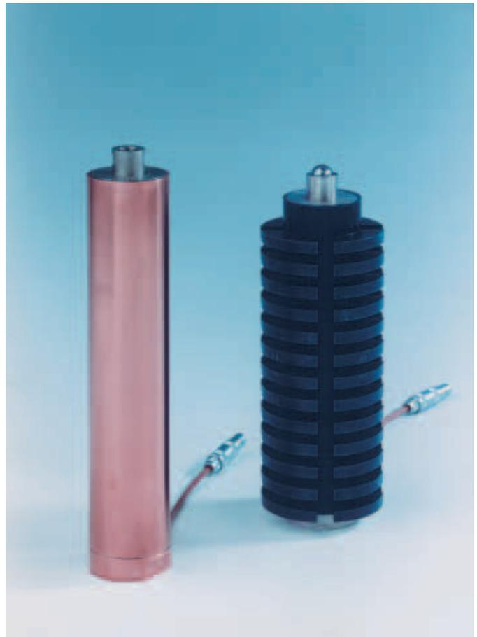
*Fig. 20: Different configurations for the heat management of actuators using the “ThermoStable” technique. Left side: actuator with copper casing for heat sinking. Right side: actuator casing with air cooling fins for forced air cooling.*
