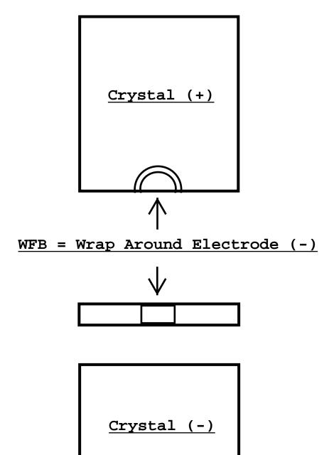
PZT Plate With WFB Wrap Around Electrode
